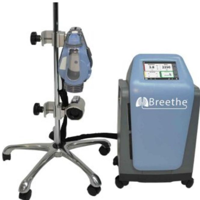
Patients who require ECMO therapy have a severe and life-threatening illness that stops their lungs from working properly. The system is connected to patients through tubes (cannulae) and is an external respiratory assistance device that takes venous blood, removes carbon dioxide and adds oxygen, much like a human lung. Oxygenated blood is then sent back to the patient. Each year, more than 20,000 patients receive ECMO therapy in the United States.
